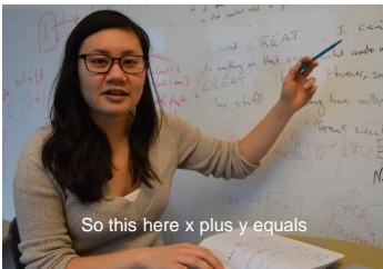
Figure 1b. Prototype 2: AR Subtitles displays one caption window that is placed at a fixed distance in front of the user and moves with user's head.
